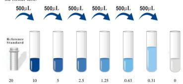
Biotinylated Detection Ab working solution: Calculate the required amount before the experiment (100 μL/well). In preparation, slightly more than calculated should be
